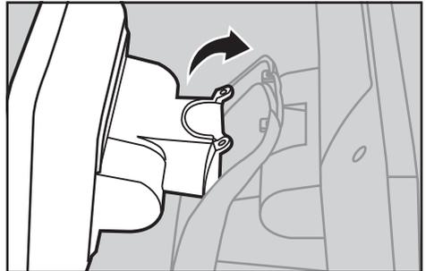
9. Fasten the customer display to the mounting points of the stand (F) using the 2 mounting screws. Make sure that the mounting screws are hand-tightened.
